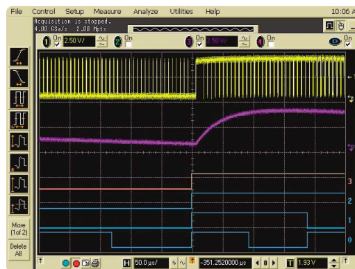
Figure 15. With the Agilent E5850A time-correlation fixture, you can make time-correlated measurements between an Agilent logic analyzer and oscilloscope.
