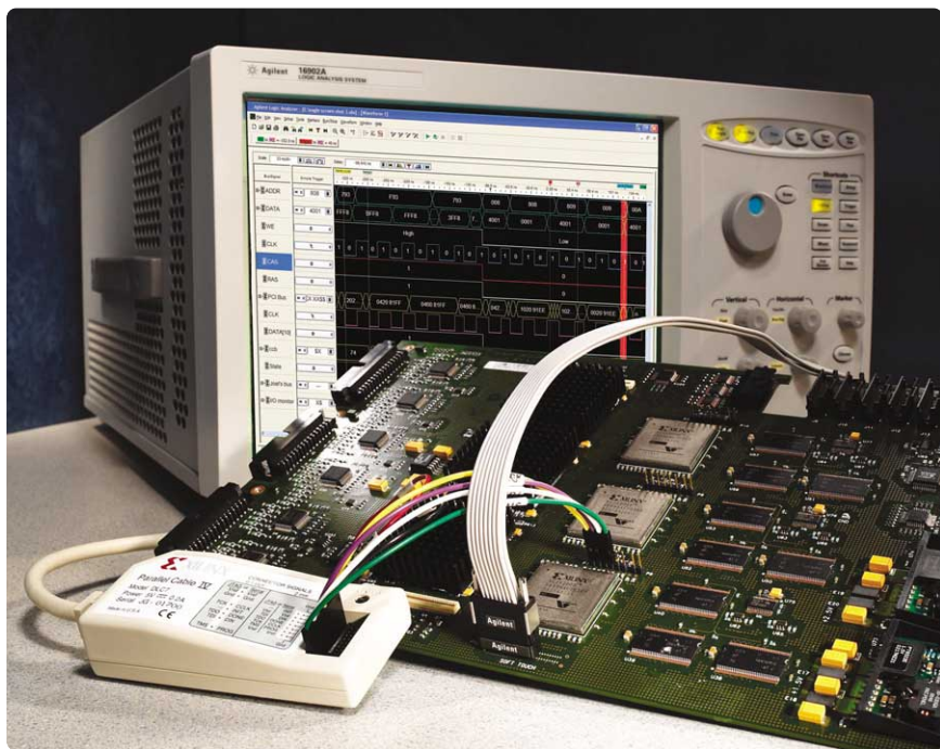
Figure 8. The FPGA dynamic probe dramatically increases debug productivity.
